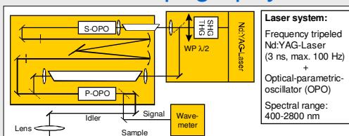
SHG/THG: Second/third harmonic generation, OPO: Optical-parametric oscillator, S/P-OPO: Seed/power OPO, WP: Waveplate, U: DC sourcemeter, MC: Monochromator, PM: Photomultiplier, CCD: Camera, PC: Computer
