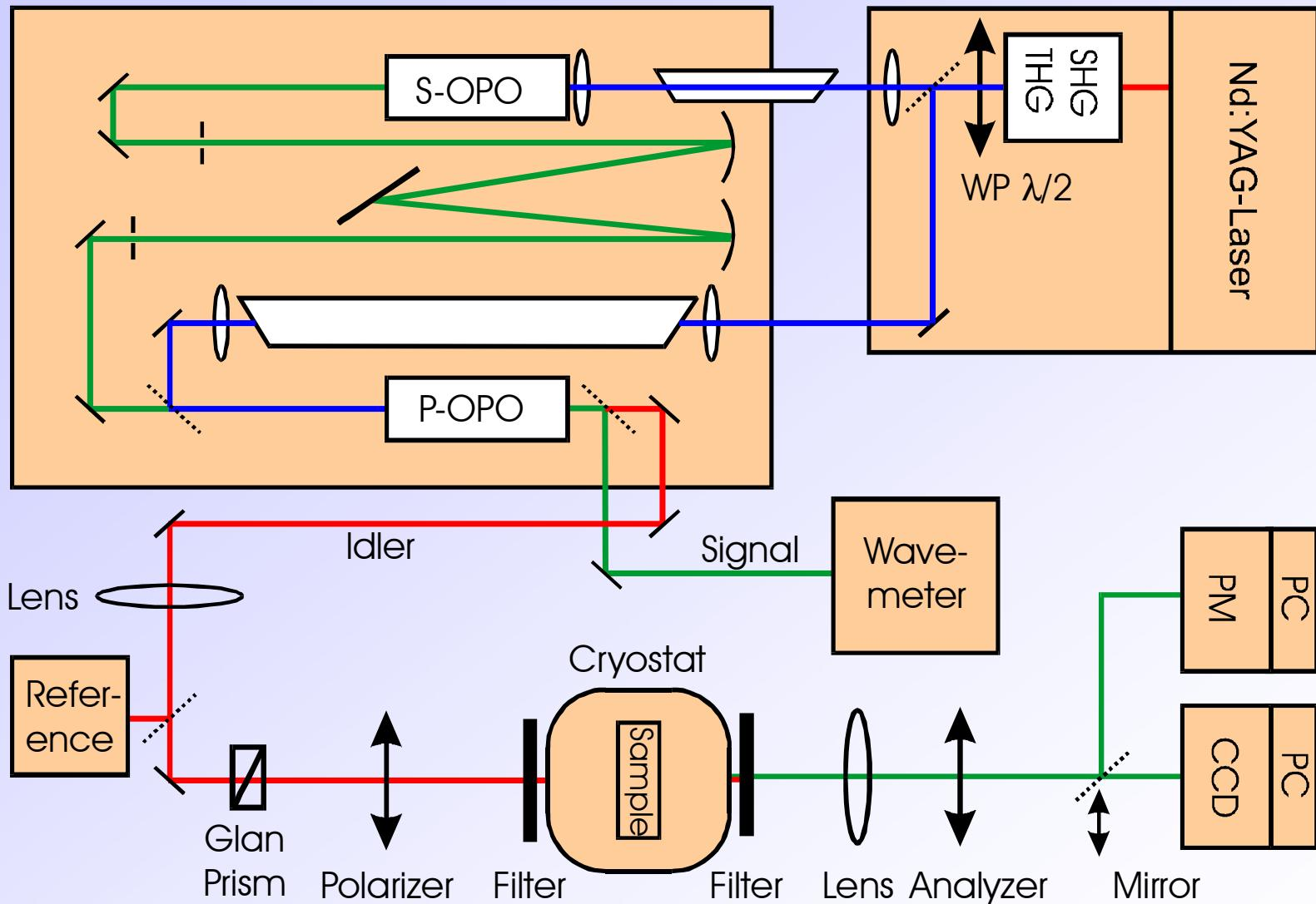
Basic setup with a pulsed Nd:YAG - OPO laser system (3 ns,  $\leq 100$  Hz, 0.4 - 3.0 mm)
